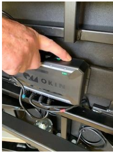
5. Pairing Press Remote Control PAIR button until blue light is flashing Press Remote PAIR button twice
